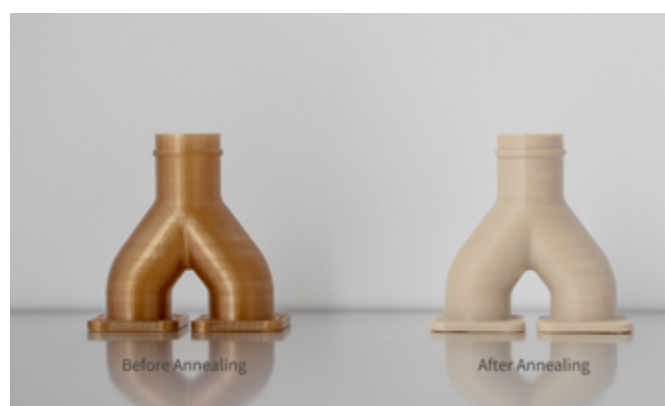
Figure 8: Manifold printed with VICTREX AM 200 filament, before and after annealing (Photo courtesy of Intamsys).
