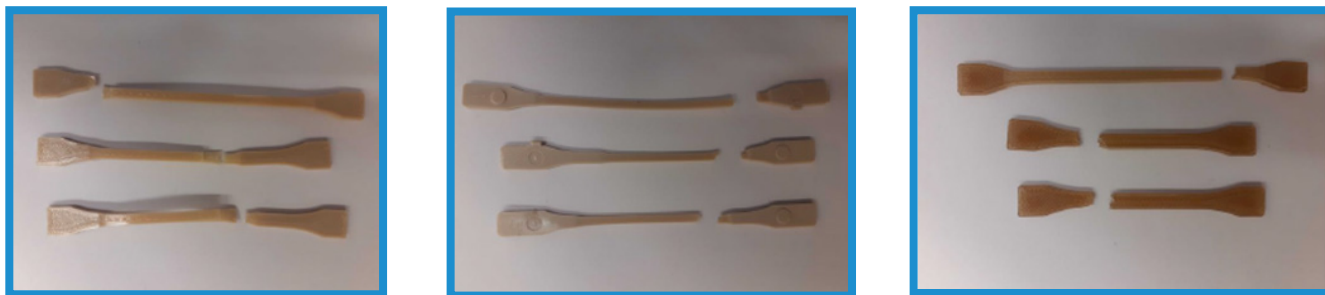
Figure 1. ISO527-2-1BA bars in Injection moulded LMPAEEK (left), VICTREX AM™ 200 printed crystalline (centre) and printed amorphous (right)
