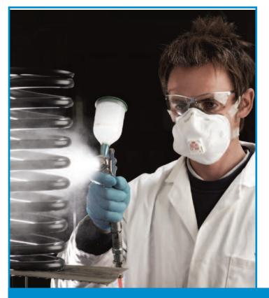
4 Apply the dispersion until an even wet surface is achieved. HVLP guns have proved effective with tip sizes of between 0.7mm and 1.8mm.
