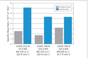
In thrust waster tests performed under different PV conditions, VICTREX HT exhibited as little as 1/3 the wear of VICTREX 450G. VICTREX HT showed a lower specific wear rate than VICTREX 450G under all other test conditions.
