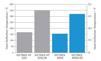
The heat deflection temperature of VICTREX HT is 13°C (23°F) higher than VICTREX 450G. When reinforced with 30% glass fiber, the HDT is 30°C (54°F) higher than any currently available thermoplastic.
