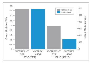
While the creep modulus of VICTREX HT and VICTREX 450G are very similar at room temperature, VICTREX HT has a creep modulus more than twice that of VICTREX 450G at 150°C (302°F). This means that VICTREX HT can support higher loads than VICTREX 450G at 150°C (302°F) without permanent deformation.
