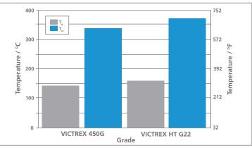
The molecular structure and semi-crystalline nature of VICTREX HT results in a melting point (T\_m) 30°C (54°F) higher and a glass transition temperature  $(T_{\alpha})$  14°C (25°F) higher than VICTREX 450G.
