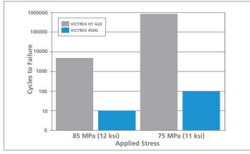
The molecular structure and semi-crystalline nature of VICTREX HT results in much better resistance to fatigue than VICTREX 450G at high levels of stress.
