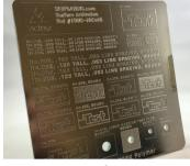
VICTREX™ PEEK plaque metallised via Surface Activation™ technology
