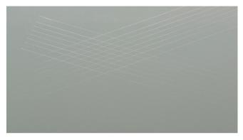
A typical scratch pattern for a Gitterschnitt adhesion test exemplifying excellent adhesion of the primer and topcoat
